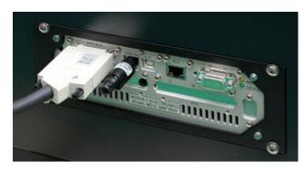
Built-in MD2i module in a Testcom machine
