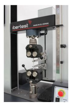
Tensile testing with a long travel extensometer. Allowing to determine elastic yield point and deformation till breaking.
